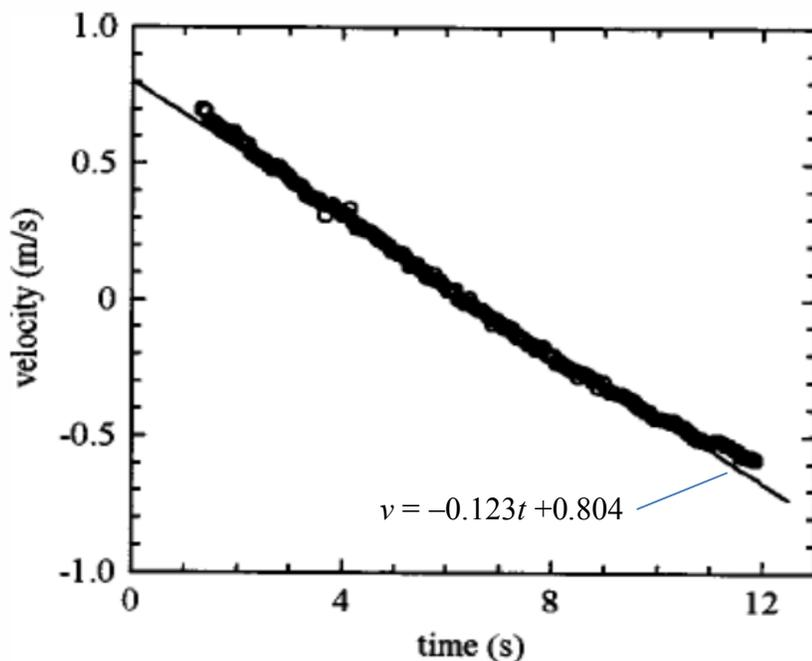
Figure 2. Velocity versus time data is shown using circles for a cart carrying a disk of radius  $r = 0.080 \text{ m}$ . The results of a linear least squares fit are also shown.
